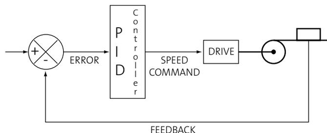
Figure 1: PID Loop
