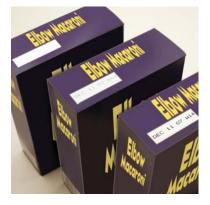
**Checking date code presence** ensures that an inkjet printer is functioning properly.
