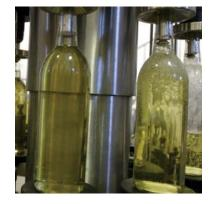
**Checking fill levels** ensures uniform product quantities, and is vital to the fill and seal process.
