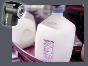
Inspection sensors are used for presence sensing, such as verifying that the cap is on and the date/lot code is present.
