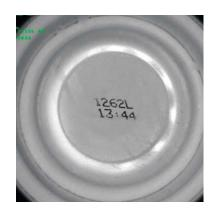
**Reading can codes** enables products to be tracked and traced through manufacturing.
